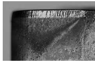
Wear on clearance face
