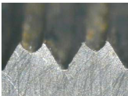
Underformed – core hole too large
