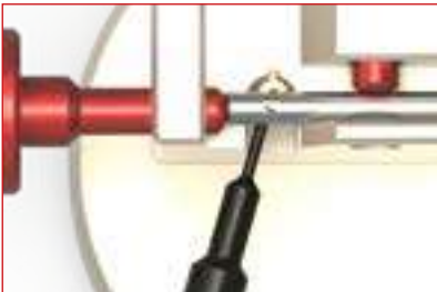
Push out the blade by using the smaller diameter of the assembly pin.
