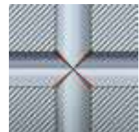
Image 3: The preloaded spring and the shaft with a recess enable the tool to deburr bores with a high degree of unevenness.
