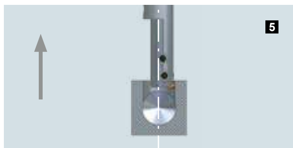
Spindle ON. Execute deburring in working feed backwards.
