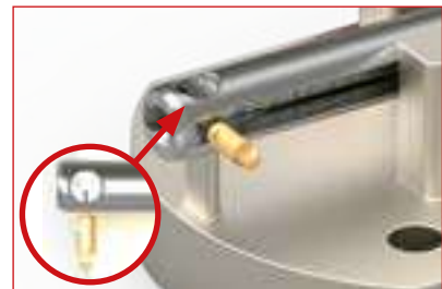
Insert new blade with cutting edges up into the blade holder. Make sure that the blade is pushed in from the line mark side.
