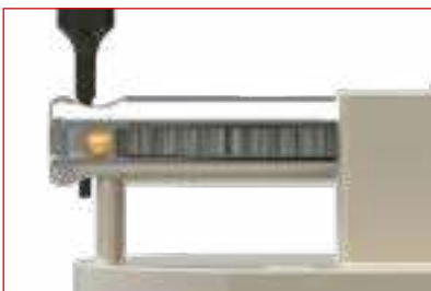
In order to define the right position of the blade and to pre-center for the new split pin, push the assembly pin in the split pin hole.
