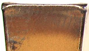
Large mechanical load produces high temperature machining, this can lead to plastic deformation.
