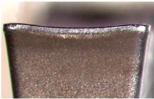
Abrasion on the flank, normal wear after a given operation time
