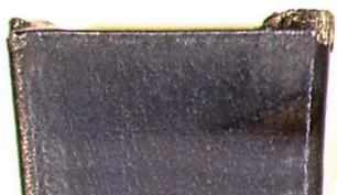
Weld deposits of material on the cutting edge occurs when the chip does not flow caused by low average temperature.
