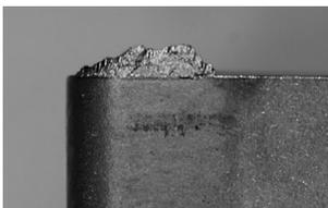
Material builds up on the cutting edge if the chip does not flow correctly due to the cutting temperature being too low.
