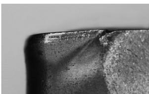
High machining temperature with simultaneous mechanical stress can lead to plastic deformation.
