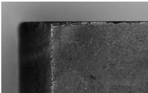
Increased mechanical stress on the cutting edge may result in carbide particles breaking off.
