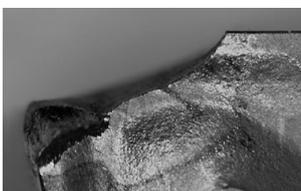
If a cutting insert is overloaded, insert breakage may occur.
