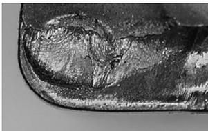
The outgoing hot chip is causing cratering of the cutting insert on the clamping surface.
